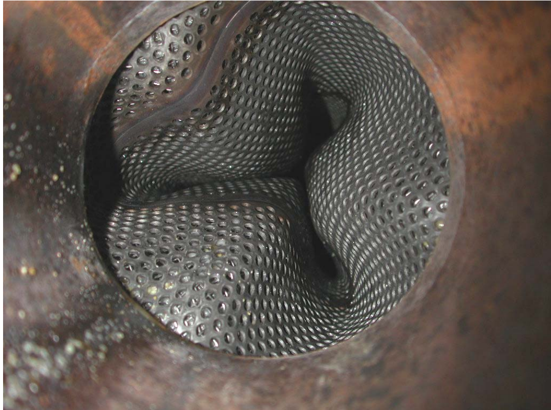
Ultimate collapse after compression test
